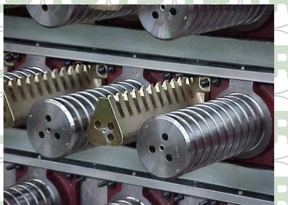
Tungsten Carbide Coating having the same composition of the UR 65 coating, but with a tighter particle structure.
